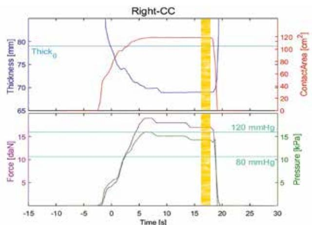
**Figure 3:** Real time recorded parameters versus time (thickness, contact area, force, pressure) during a single compression procedure. For comparison average blood pressure is indicated (80 - 120 mmHg). The vertical yellow bar indicates the image acquisition and radiation exposure
