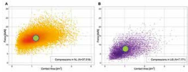
**Figure 2:** Graphical display of the range of forces between the contact area of the paddle and the breast in mammography. There is a large variation in forces applied within both the Dutch site (left panel) and the US site (right panel) and between Dutch and US sites. The green dots represent the center of the data.
