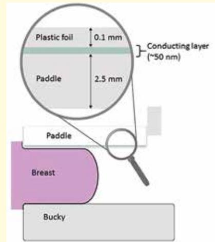
To automatically measure the contact area of the breast with the compression paddle, the Sensitive Sigma Paddle incorporates a proprietary thin (0.1mm) film containing silver nano-wires to measure capacitance. The film is fitted in the paddle and has minimal effect on X-ray transmission and scattering.
